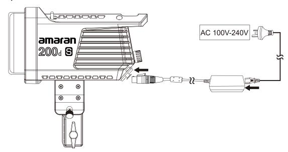
\*Please press the button on the DC interface to remove the power cord from the lamp. Do not pull it out forcibly.
