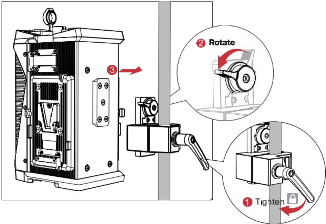
3) To remove the Control Box, grasp it firmly, and unlock the quick-release plate by rotating its lever.
