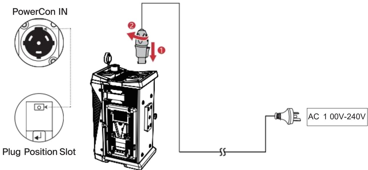
\*To disconnect the cable, pull back on the silver release tab on the cable connector, and rotate the connector counter clockwise. Do not pull directly on the cable.
