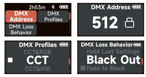
\* The fade-out time decreases as the percentage of brightness decreases. When the brightness output is 100%, the fade-out time is 60 seconds, which decreases in sequence.
